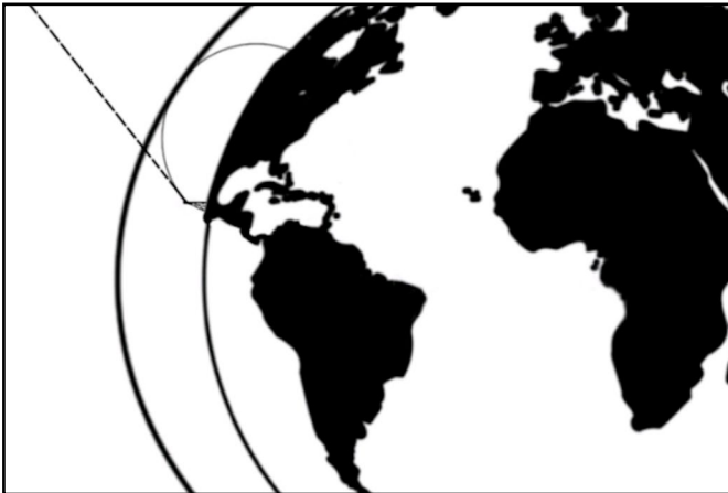
Figure 2. The diurnal skywave effect model shows the impact of the compressed ionosphere (thick solid line) on AM (thin solid line) versus FM (dashed line) signals.
